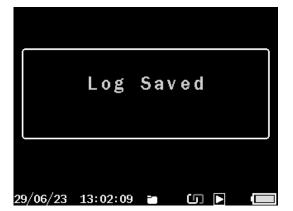
Average tests are automatically stored in memory with a log number - Send test logs to your optional KANE-IP3 printer or KANE LIVE App by pressing ENTER.
