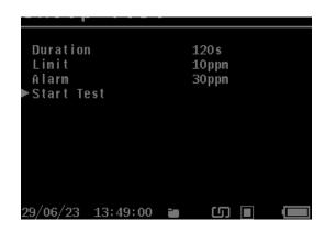
Select Setup Sweep Test to start a new test
