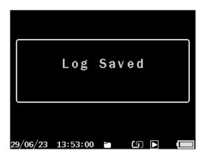
Sweep tests are automatically logged in memory with a log numbers - Send test logs to your optional KANE-IRP3 printer or KANE LIVE App by pressing **ENTER**.
