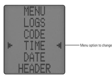
Press ▲ or ▼ to change option then press **ENTER** to confirm. To exit **MENU** rotate dial to any position - Unsaved changes will be lost.
