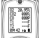
Remove the probe from the flue and allow analyzer to purge with fresh air until readings return to zero. 02 to 20.9%, CO to Zero (Be careful the probe tip will be HOT).
