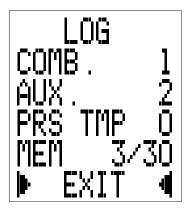
To view the current memory usage status simply navigate to menu ----> LOGS, press the ➡ button to select the Log desired.
